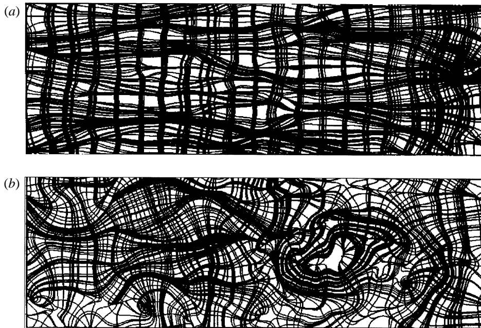
FIGURE 17. Skin-friction lines and surface vorticity lines superimposed. (a) Unseparated region. (b) Separated region.
